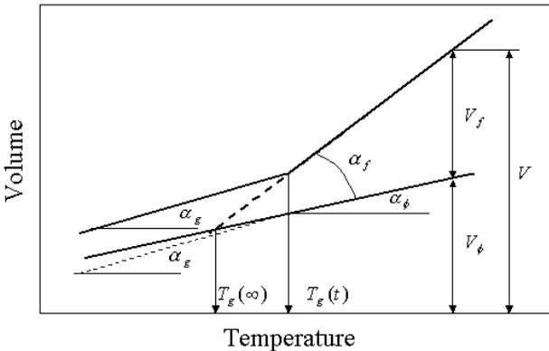
**Figure 4:** Volume-temperature diagram of an amorphous polymer.
