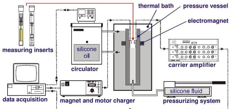
**Figure 10.** Schematic of the CEM Measuring System [1, 62].
